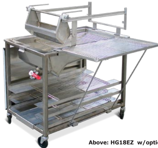
Above: EasyLift glazer in operation, showing sliding glaze applicator
